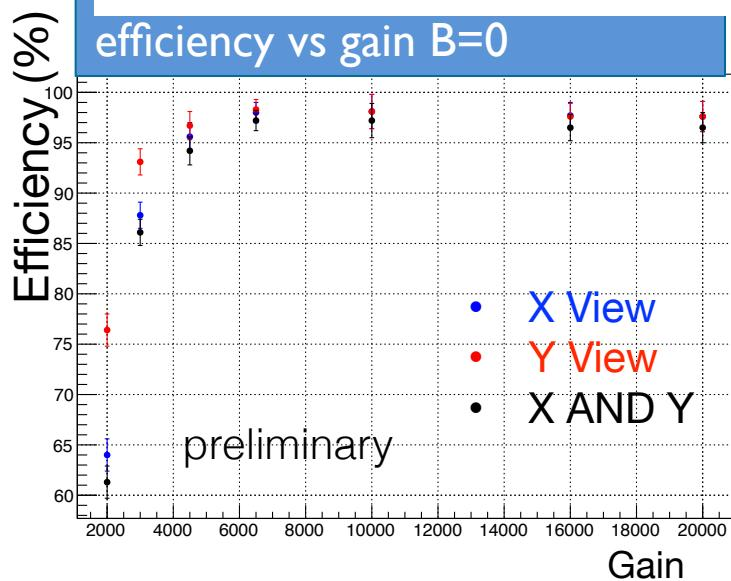
With Ar/Isob (90/10) gas mixture, 650  $\mu\text{m}$  strip pitch, 3mm gap, B=0 :
