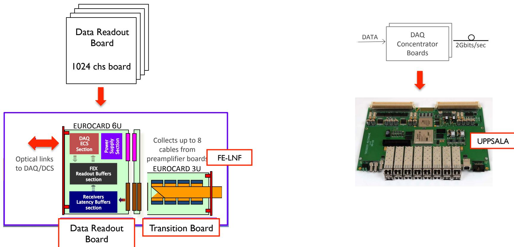
Readout Boards must match the **ASICs data driven** architecture with **BES DAQ based on LI trigger** and **6.4 (nominal) latency time**
