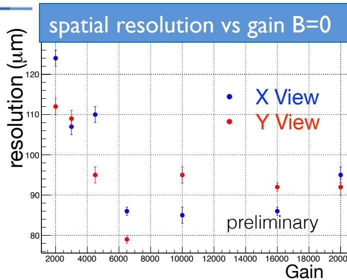
With Ar/Isob (90/10) gas mixture, 650  $\mu\text{m}$  strip pitch, 3mm gap, B=0 :
