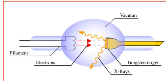
The *Coolidge tube* (1913), also called *hot cathode tube*, is the most widely used. Electrons are produced by thermionic effect from a tungsten filament heated by an electric current. The filament is the cathode of the tube. The high voltage potential is between the cathode and the anode, the electrons are accelerated, and hit the anode.
