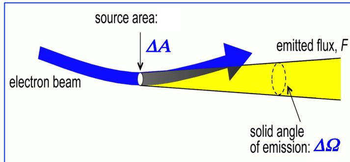
In a storage ring the *product of the electron beam transverse size* and *angular divergence* is a constant along the ring and is called *emittance* (*vertical* and *horizontal emittance*).
