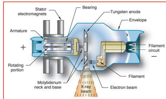
The *rotating anode tube* is an improvement of the *Coolidge tube* anode surface (water cooled) is always moving, so heat is spread over a much larger surface area giving a 10-fold increase in the operating power.
