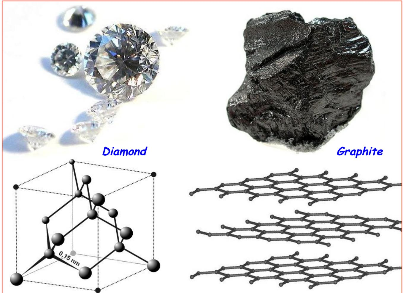
In *graphite*, the *individual carbon atoms link up to form sheets of carbon atoms*. Within each sheet every carbon atom is bonded to three adjacent carbon atoms (*covalent bonds*) producing hexagonal rings of carbon atoms. *Weak bonding forces called van der Waals forces hold the sheets together*. Because these *forces are weak, the sheets can easily slide past each other*. The sliding of these *sheets gives graphite its softness for writing and its lubricating properties*.
