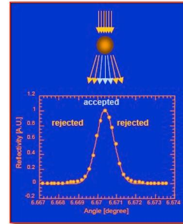
**Diffraction Enhanced Imaging (DEI) or Analyzer-Based Phase-Contrast Imaging (ABI-PCI)** is based on the use of *a perfect crystal analyzer crystal placed between the sample and the imaging detector.*
