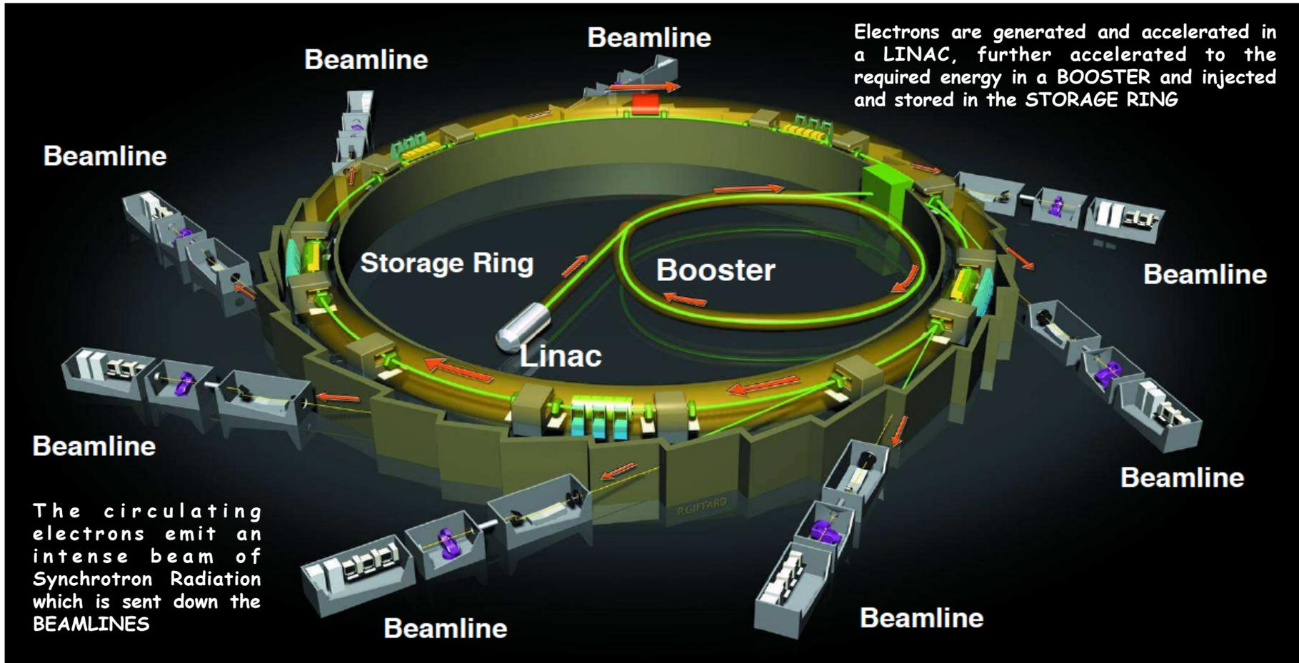
As a function of the energy range to be used each beamline must be optimized for a particular field of research.
