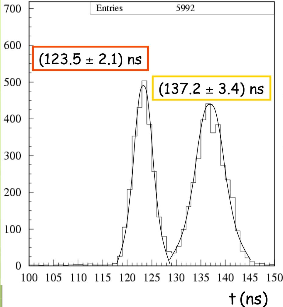
$$t_{12} = \bar{t}_2 - \bar{t}_1 = 13.7 \text{ ns}$$
