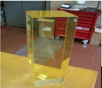
The lead glass is the medium in which the Cerenkov effect occurs. It is made basically by a mixture of lead and glass, so that in this material the speed of the light is smaller than the particle's one, giving the Cerenkov effect.
