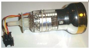
The Photomultiplier tubes (PMT) are extremely sensitive detectors of light in the ultraviolet, visible and near infrared. These detectors multiply the signal produced by incident light by as much as 10<sup>8</sup> from which single photons can be resolved.
