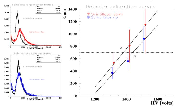
To create the curve of calibration we plotted the gains of the three measurements at three different voltages in a Cartesian system. We did a fit in order to find the calibration curve of each scintillator, then we choose a gain fixing the voltage at the value that we found (point A = 1381 volt; point B = 1440 volt).
