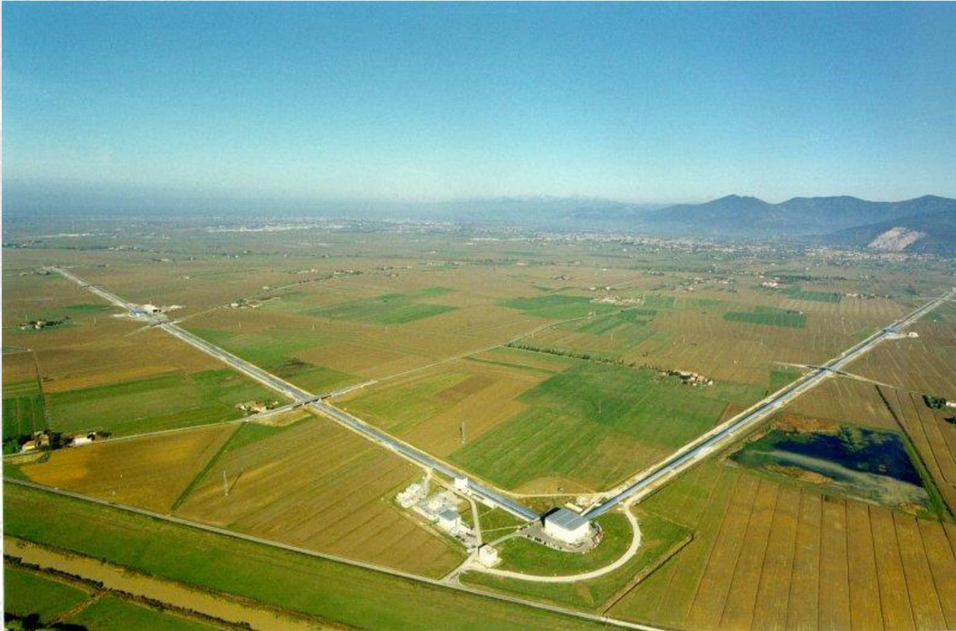
The effect of the GW is proportional to the length of the interferometer arms → long arms are needed (3 km)
