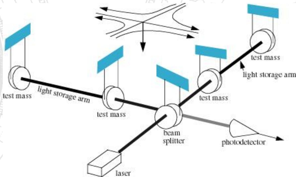
*Also with  $L=3\text{ km}$  the displacement of the mirrors is  $3 \times 10^{-18}\text{ m}$ :
