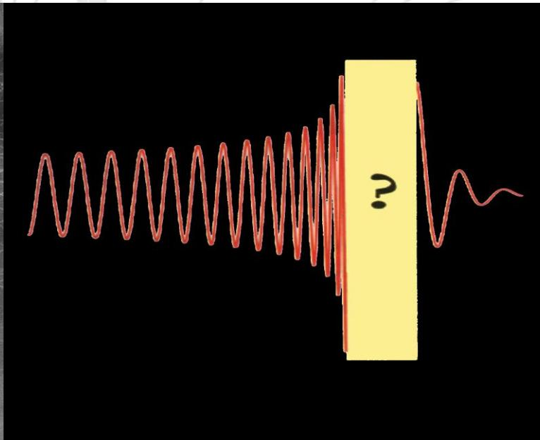
The signal emitted has a very characteristic shape called chirp
