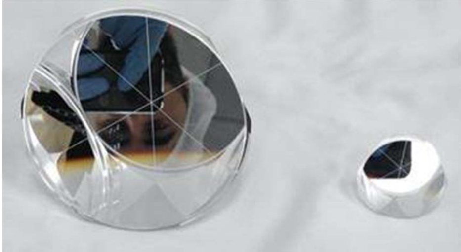
The 2nd generation retroreflector developed by LNF and University of Maryland (left) next to a 1st generation Apollo reflector (right)
