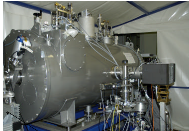
Stretched wire field measurement (integral measurements)
