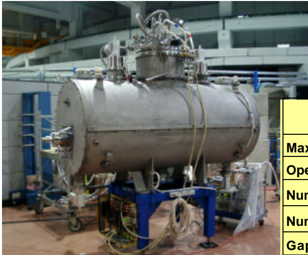
3.5 TESLA SUPERCONDUCTING WIGGLER for ST (TRIESTE, Italy), 2002
