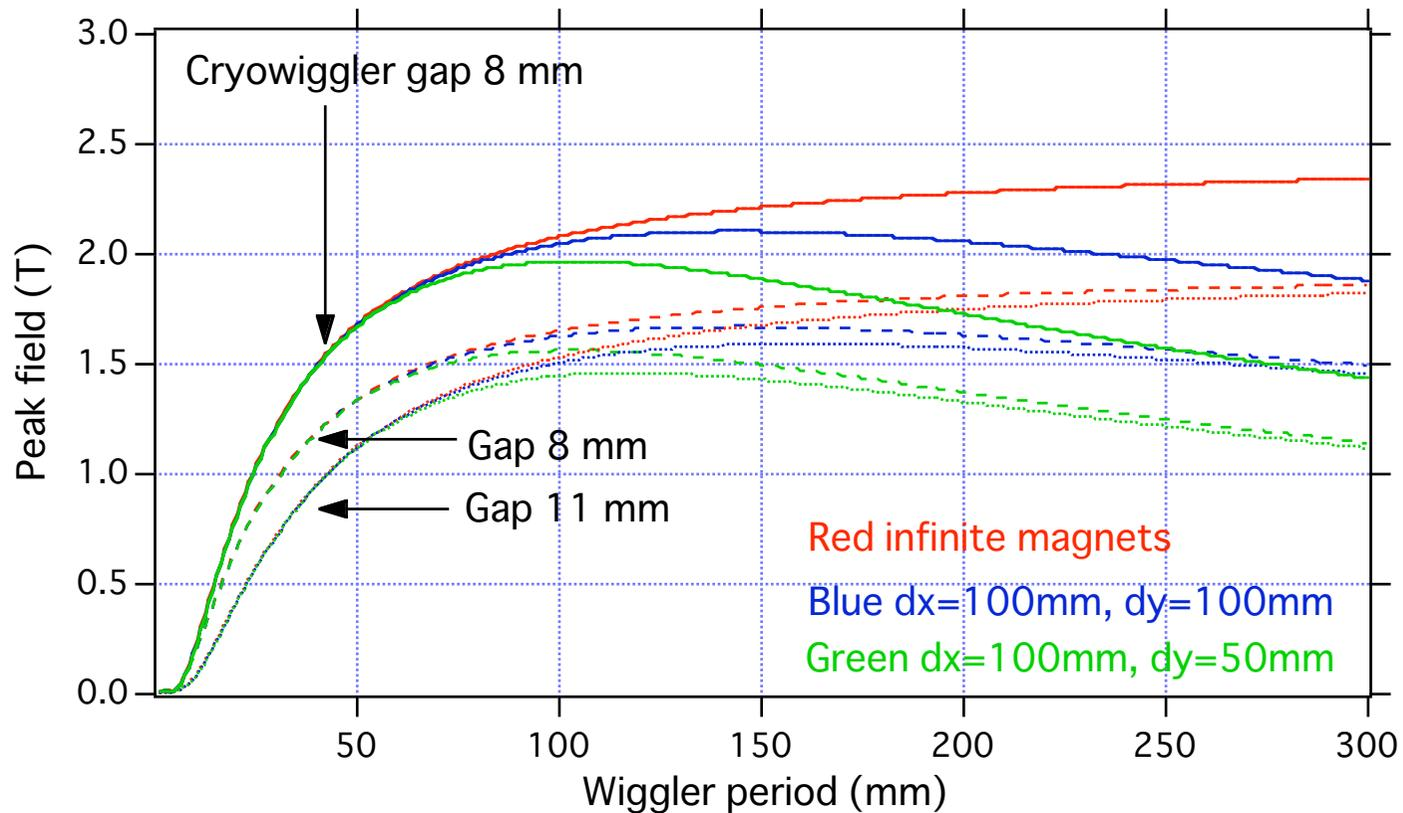
Peak fields of **pure magnet type wigglers**, cryogenic wiggler (solid lines), in-vacuum wiggler (dashed lines) and out of vacuum wiggler (dotted lines).
