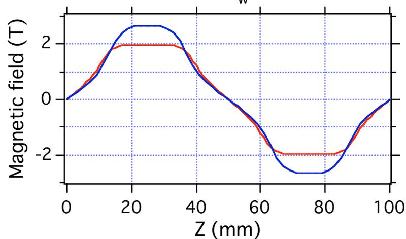
PPM cryowiggler gap=8 mm,  $\lambda_w=100$  mm
