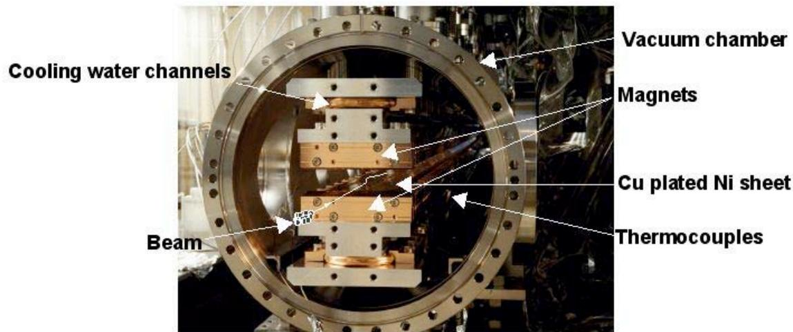
Cross section of in-vacuum device
