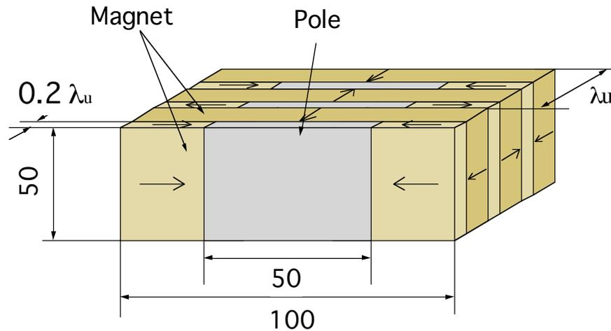
Hybrid structure for high field wiggler.
