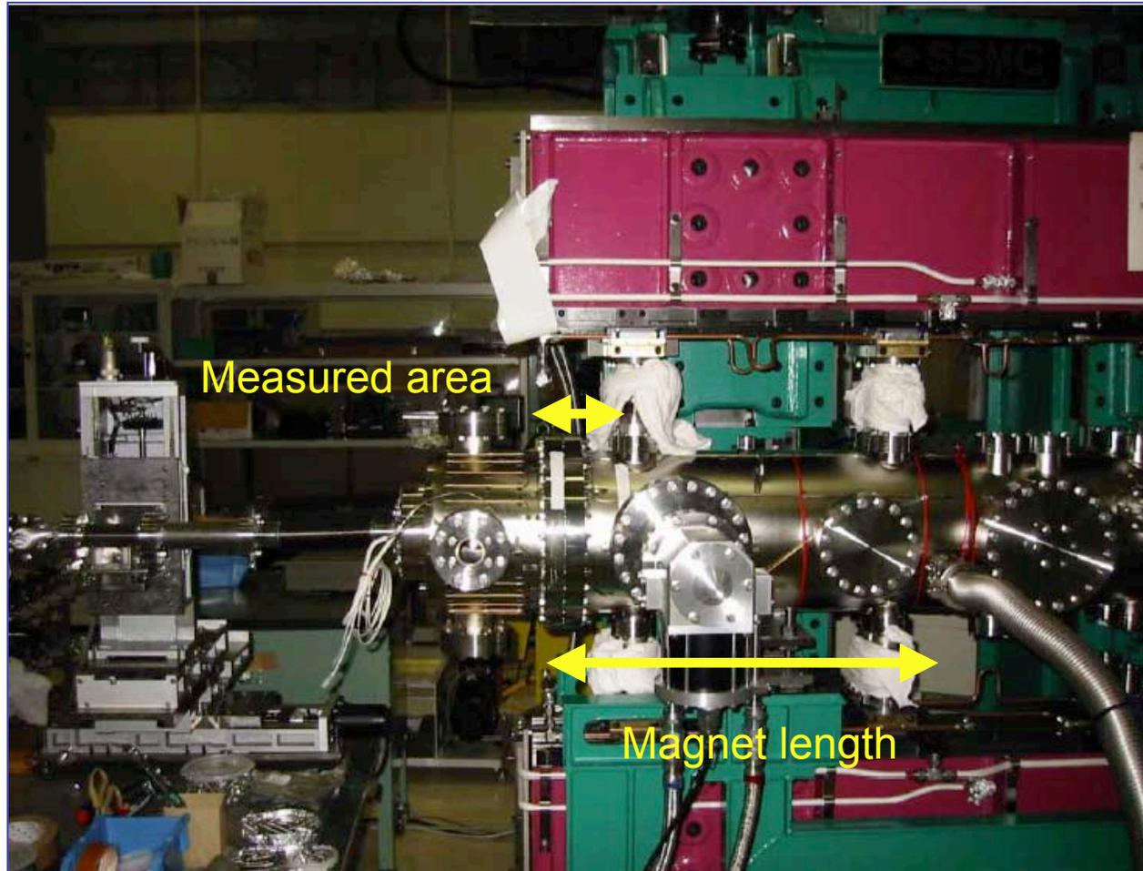
Field measurement using a hall probe in vacuum at 5 mm gap.
