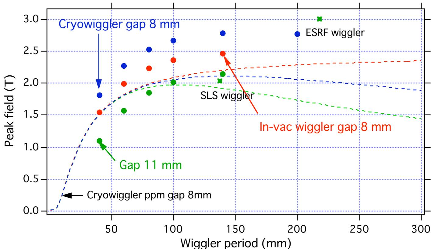
Peak fields of **hybrid type wigglers**, cryogenic wiggler (blue circles), in-vacuum wiggler (red circles) and out of vacuum wiggler (green circles), dashed lines are ppm cryowiggler for comparison.
