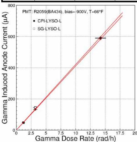
γ-ray induced PMT anode current can be converted to the photoelectron numbers (Q) integrated in 100 ns gate. Its statistical fluctuation contributes to the readout noise (σ).
