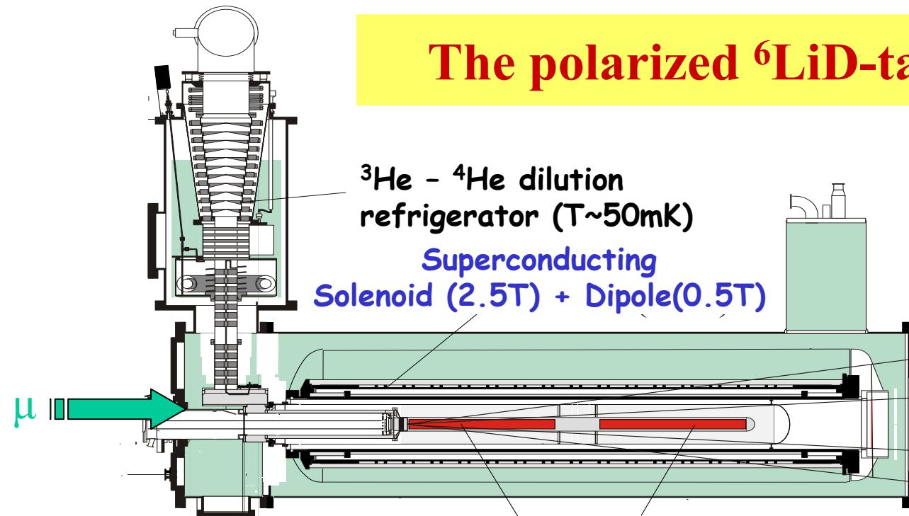
Two 60cm long target cells with opposite polarizations
