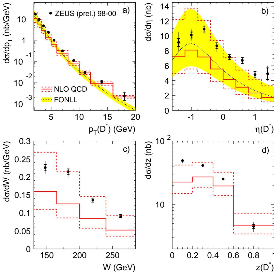
$z(D^*)$ : Photon energy fraction carried by  $D^*$  in  $p$  rest frame
