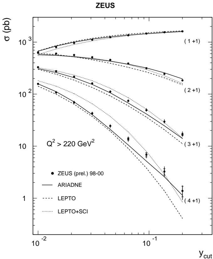
**ZEUS plot 3-jet cross section vs  $y$  jet separation parameter**
