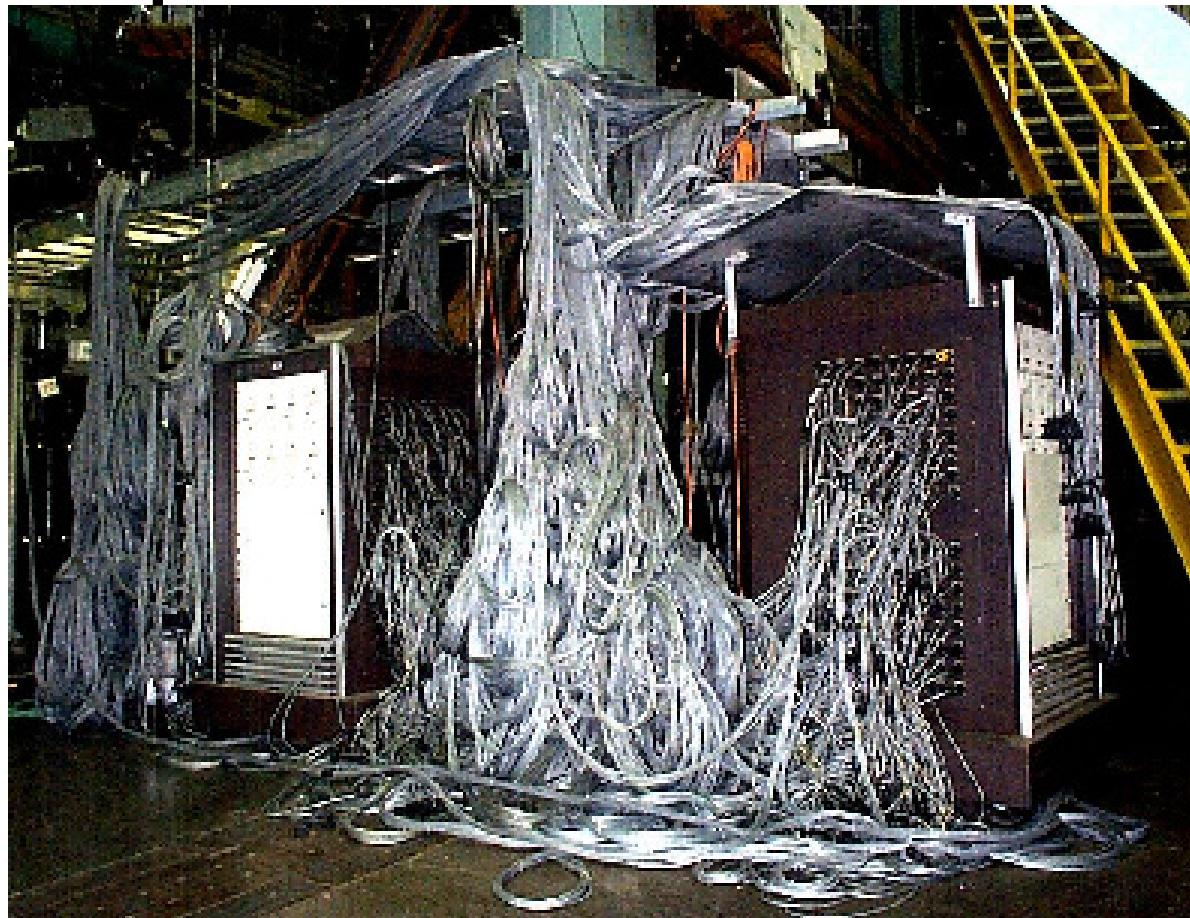
**F-18 Aircraft Static Fatigue Test System**
