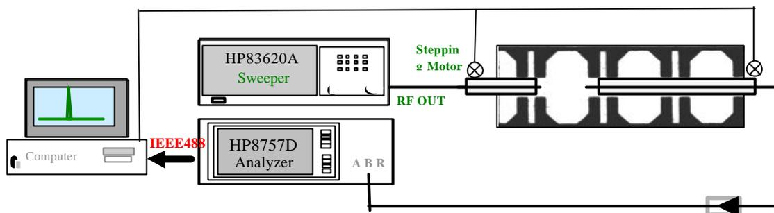
Fig.1 Cavity properties measuring
