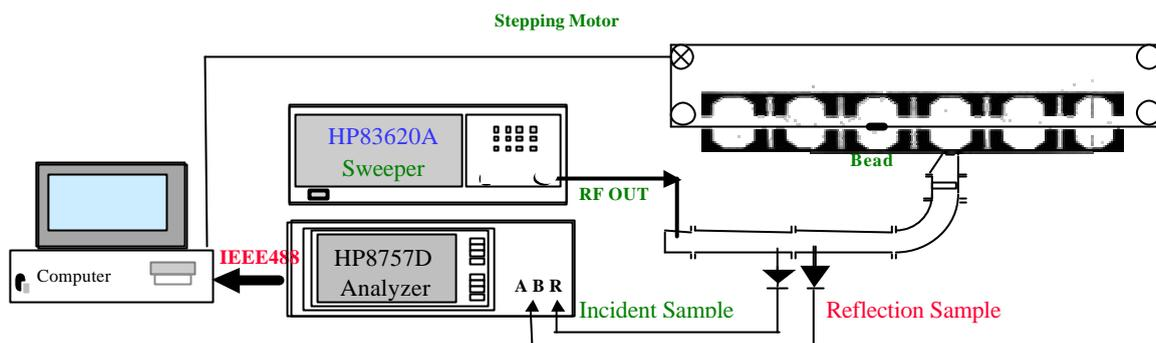
Fig.2 Axial electric field distribution measuring
