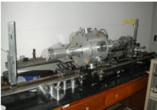
Fig.5 Disturbing bead with the thread and supporters
