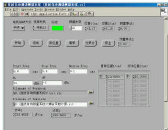
Fig.7 Cavity properties measuring interface
