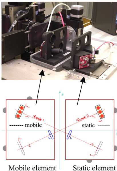
Figure 3: The Praxial system (bottom) and the Praxial sensor installed on the Caliprax calibration bench (top).
