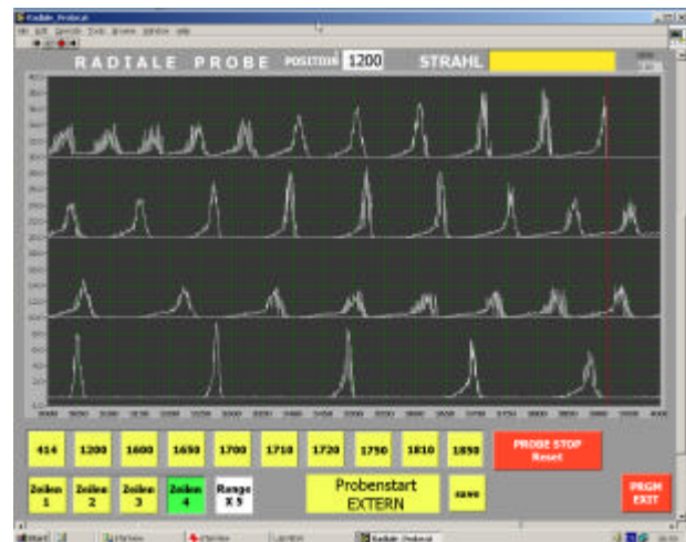
Fig 6: A C-programmed LabVIEW VI-library allows standardised remote access to parameters of the main VISTA control system. This example is part of the ISL control system illustrating the turn-pattern acquisition of a beam in the ISL cyclotron by moving a differential radial probe.
