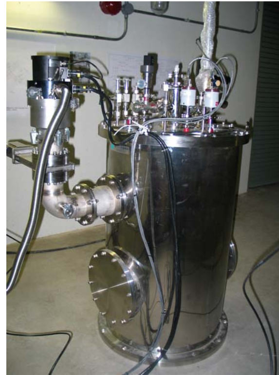
Test cryostat at MTA
