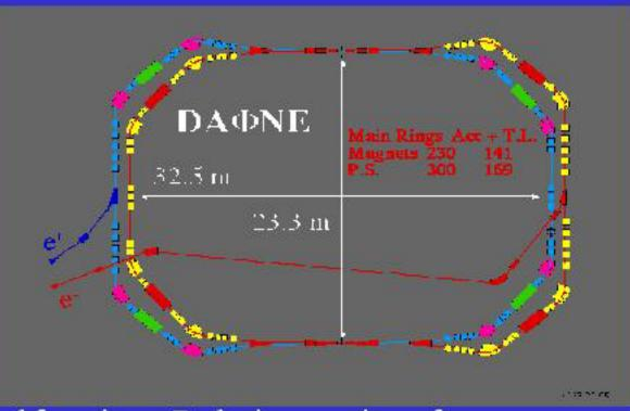
structure and the same optical functions. Each ring consists of two symmetric parts which have similar structure: an inner one named "short" and an outer one named "long". Photon beams for SR applications will be extracted by the 'long' arc section. The sources planned for this application are one wiggler and two bending magnets.
