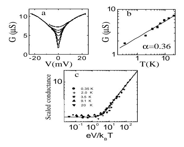
Scaling plot for  $T^{-\alpha}dI/dV$  vs.  $eV/k_BT$  very similar to Luttinger liquid!
