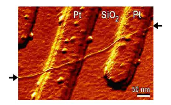
Fermi (doping) level tunable, e.g. using gate voltage
