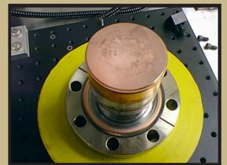
Damage appears as a ring on the surface where maximum heating has occurred.
