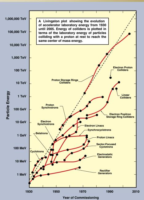
The Livingston curve shows the exponential growth in CM energy that has come from new accelerator physics and technology. This growth has been followed by profound discoveries — CP violation in K s, two v s, J, quarks,  $\Psi$ ,  $\tau$ , gluons and QCD, W, Z, top quark. The ORION center would directly address crucially important new accelerator ideas.
