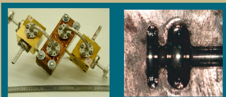
Major RF components of the W-Band Photoinjector are shown in the above photographs. The Zipper W-Band Traveling Wave Accelerator (left), and the W-Band RF Gun (right), both provide excellent examples of the results of the synergistic relationship between SLAC and small business as they work together through the U.S. Department of Energy Small Business Research Initiative (SBIR) Program in the field of advanced accelerator research.
