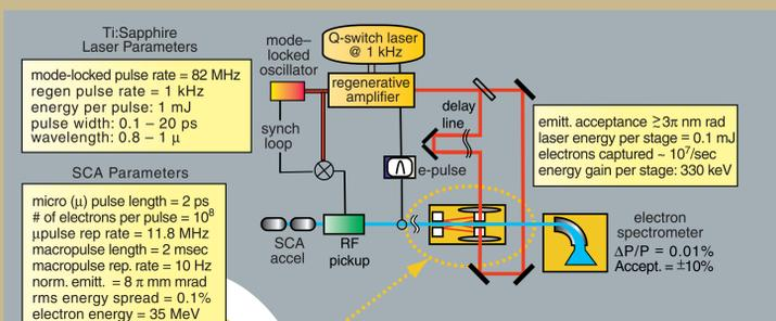
SLAC and Stanford are collaborating on the laser acceleration work described in the adjoining figures. HEPL SCA is used to produce low transverse and longitudinal emittance electron bunches that are analyzed with a high resolution spectrometer.
