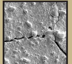
Damage in the form of cracks and grain growth after 55 million pulses at 120 degrees C pulsed temperature increase is shown.
