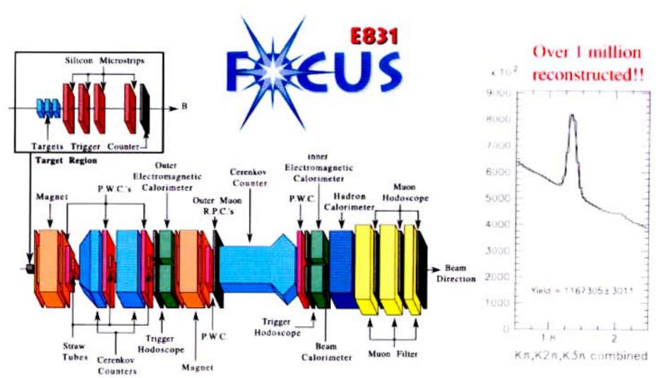
Successor to E687. Designed to study charm particles produced by ~200 GeV photons using a fixed target spectrometer with upgraded Vertexing, Cerenkov, E+M Calorimetry, and Muon id capabilities. Includes groups from USA, Italy, Brazil, Mexico, Korea
