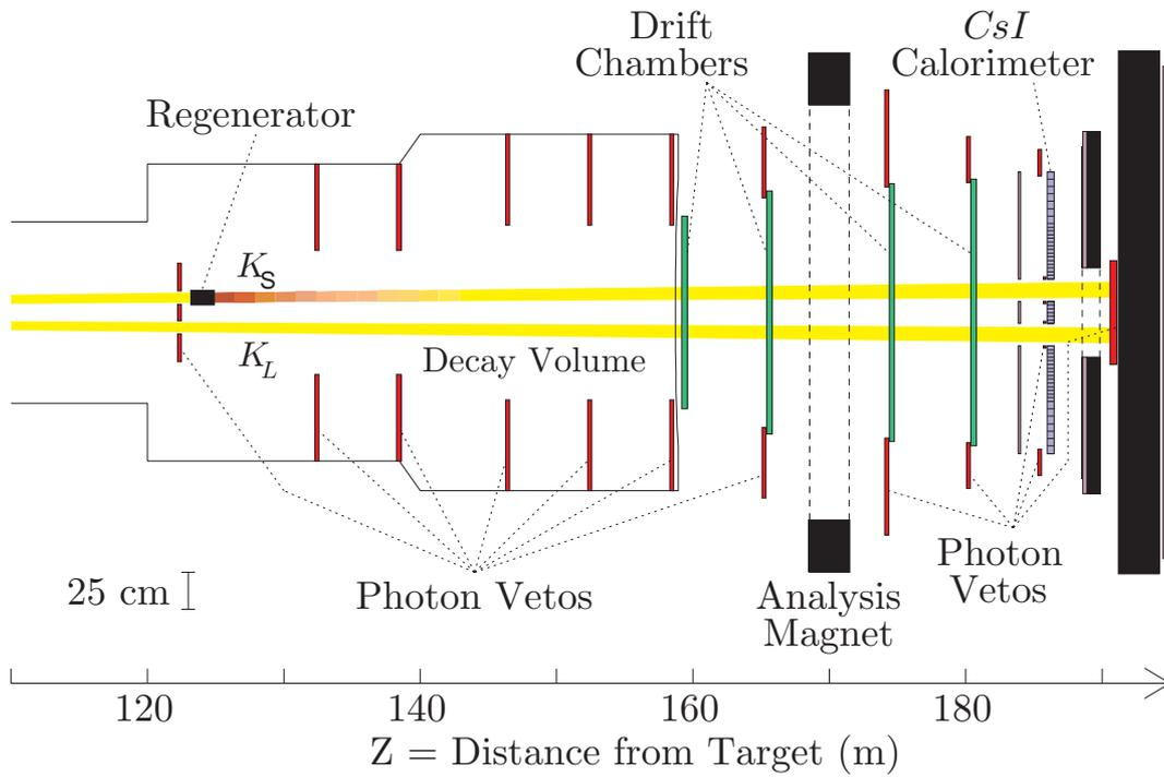
Fig. 17. Plan view of the KTeV experiment. Note the different scales.
