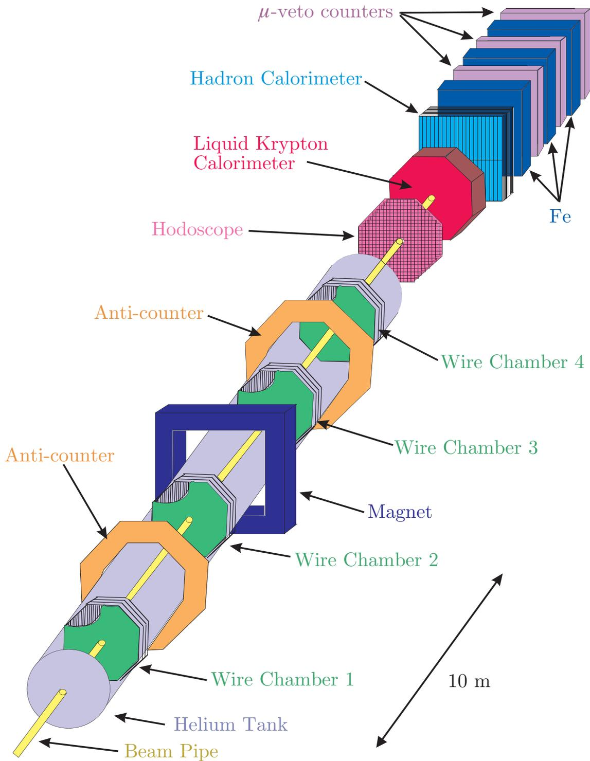
Fig. 16. The NA48 experiment at CERN
