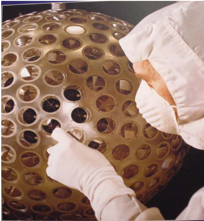
Laser Geodynamic Satellite Experiment (LAGEOS) LAGEOS satellites reflect laser beams transmitted from ground stations back to sensors on Earth.
