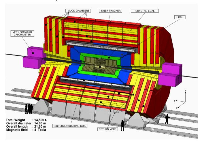
CMS Compact Muon Solenoidal Detector for LHC
