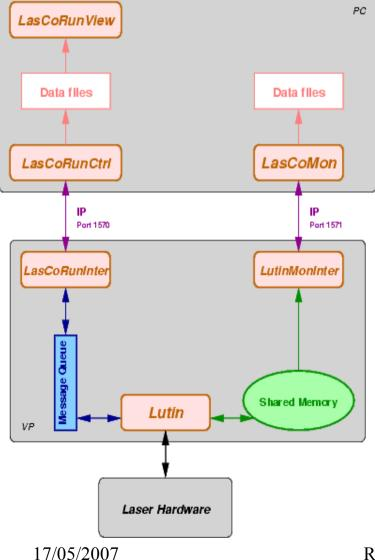
LasCo (for Laser Controller) is a graphical user interface dedicated to the monitoring and the standalone running of the TileCal Laser System. In this particular environment, standalone means without any input from the official Atlas DAQ or DCS. Therefore, it is intended to be used during the Laser System commissionning, as well as during the future maintenance periods.
