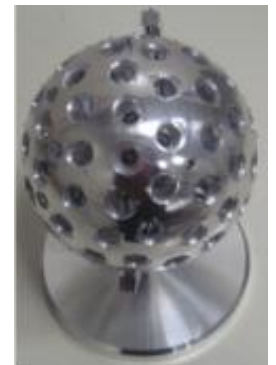
Figure 2: the INFN-LNF DSGP test mass
