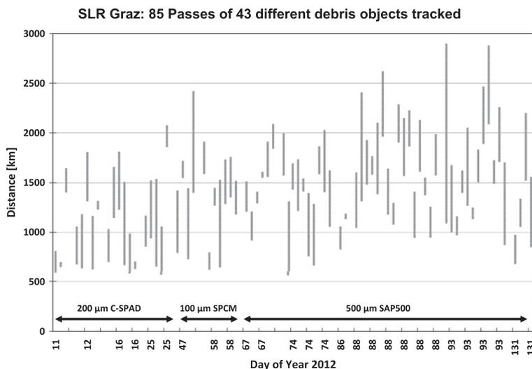
Fig. 2. Graz Debris Ranging Results: 85 successfully tracked passes, with objects in distances from 600 km up to more than 2500 km. Detectors with different diameters were used:  $200 \mu\text{m}$  C-SPAD,  $100 \mu\text{m}$  SPCM (Single Photon Counting Module, of Micro Photon Devices),  $500 \mu\text{m}$  SAP500.
