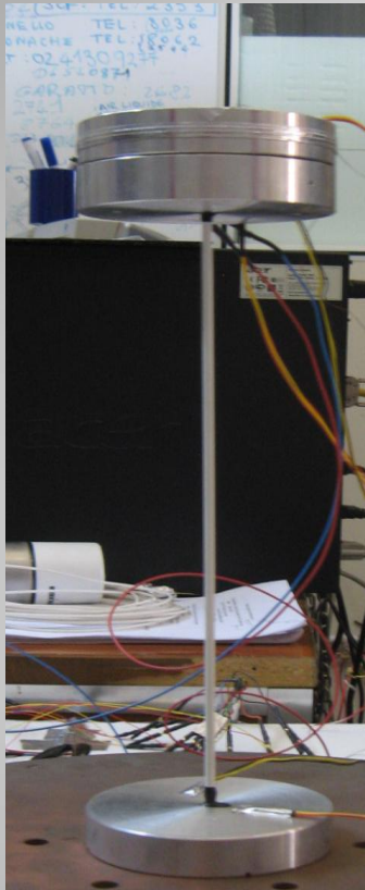
Breadboard for thermal interface study between CCR and mounting rings
