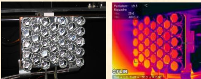
Third GPS flight array inside the SCF (left) and an IR thermogram taken during Solar Simulator illumination (right).
