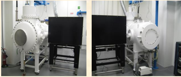
Front and rear view of SCF cryostat. Optical instrumentation is in the black enclosure.
