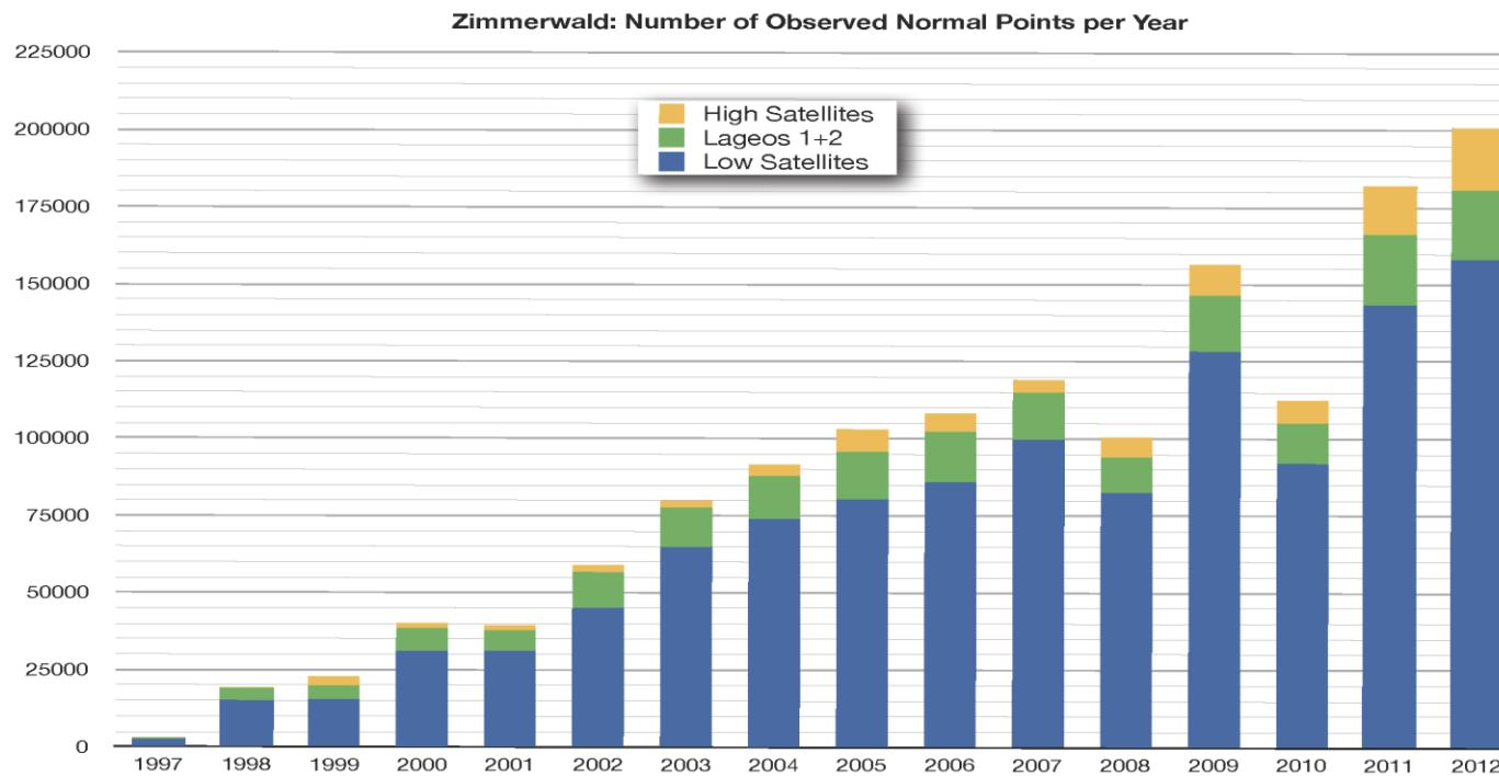
Minor improvements in the number of observed NPs/Year for GNSS satellites, increasing number can be seen for all type of satellites (LEOs, LAGEOS, GNSS) due to improvements in the steering of the rotating shutter.
