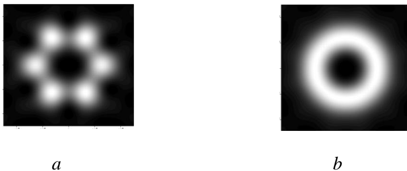
Fig.1 Far field diffraction patterns (FFDP) of reflected light from a single CCR with interference coating (a) and from retroreflector array (b)
