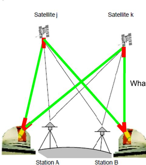
Fig. 2. SLR double-differences (green) with satellite biases and station range biases (red).
