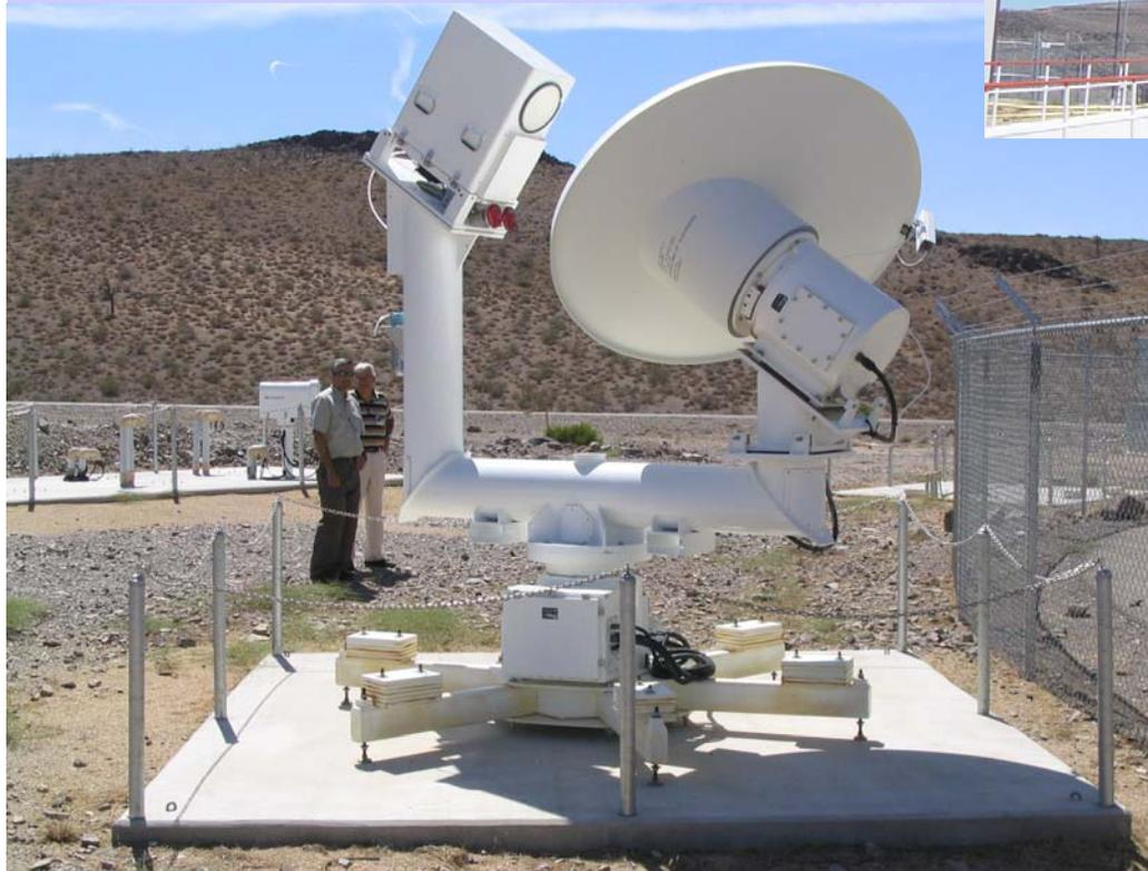
**The Advanced Media Calibration System for tropospheric dry and wet path delay corrections.**
