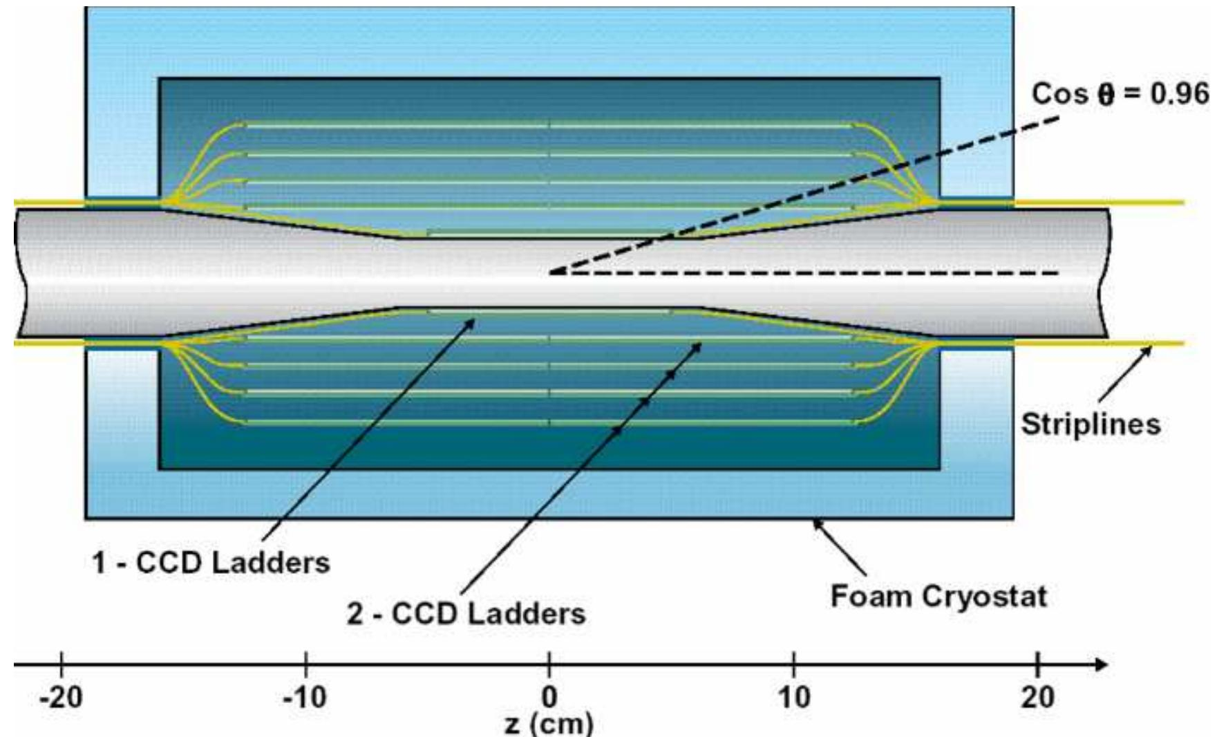
5 CCD layers at 15, 26, 37, 48 and 60 mm. Each layer  $< 0.1\% X_0$ .
