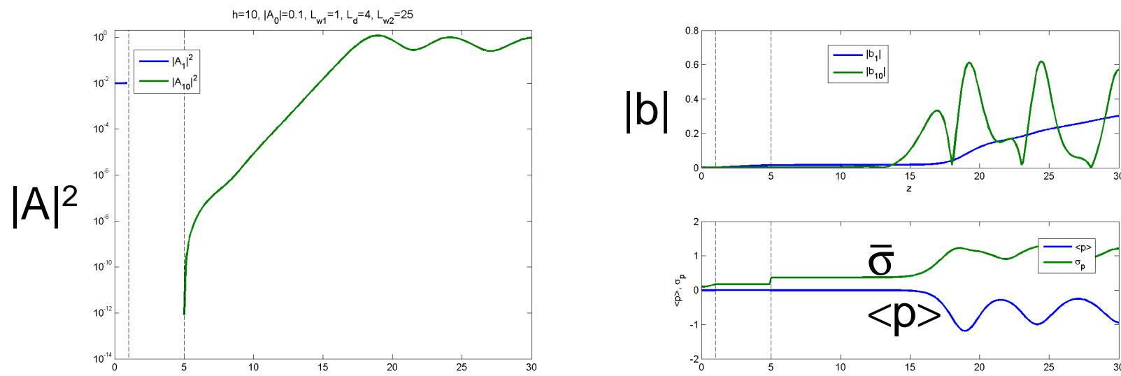
Drift section ( $\bar{L}_d=4$ ) has increased harmonic intensity by 2 orders of magnitude
