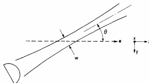
FIG. 1. The electrons move in the  $z$  direction and the wave is propagating at an angle  $\theta$  to this direction. It is assumed that the field can be represented by a plane wave in the interaction region, with the field vector polarized in the  $yz$  plane. A cylindrical lens is used so that there is little variation in field intensity in the  $x$  direction.
