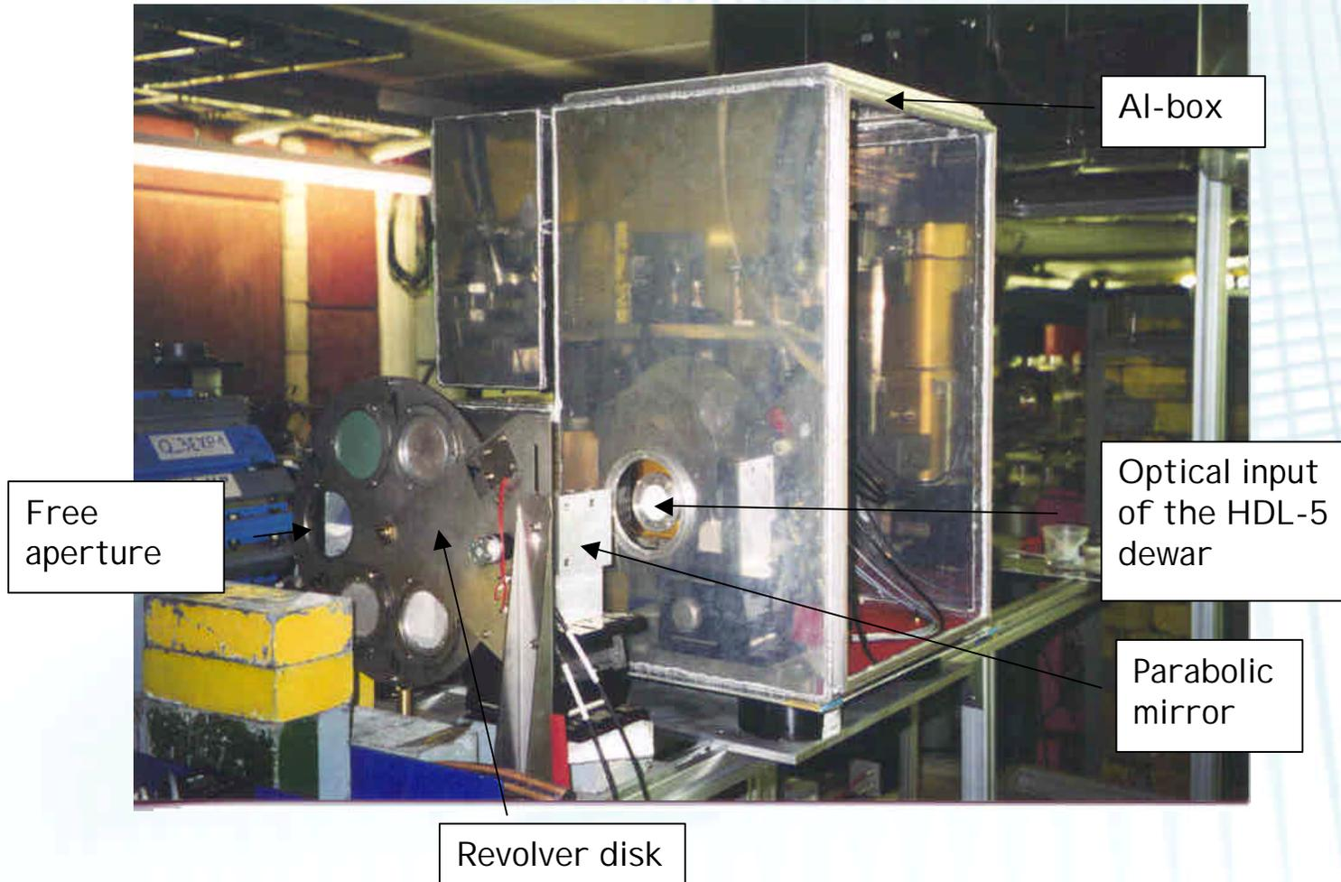
The view of the HT spectrometer from the optical input.
