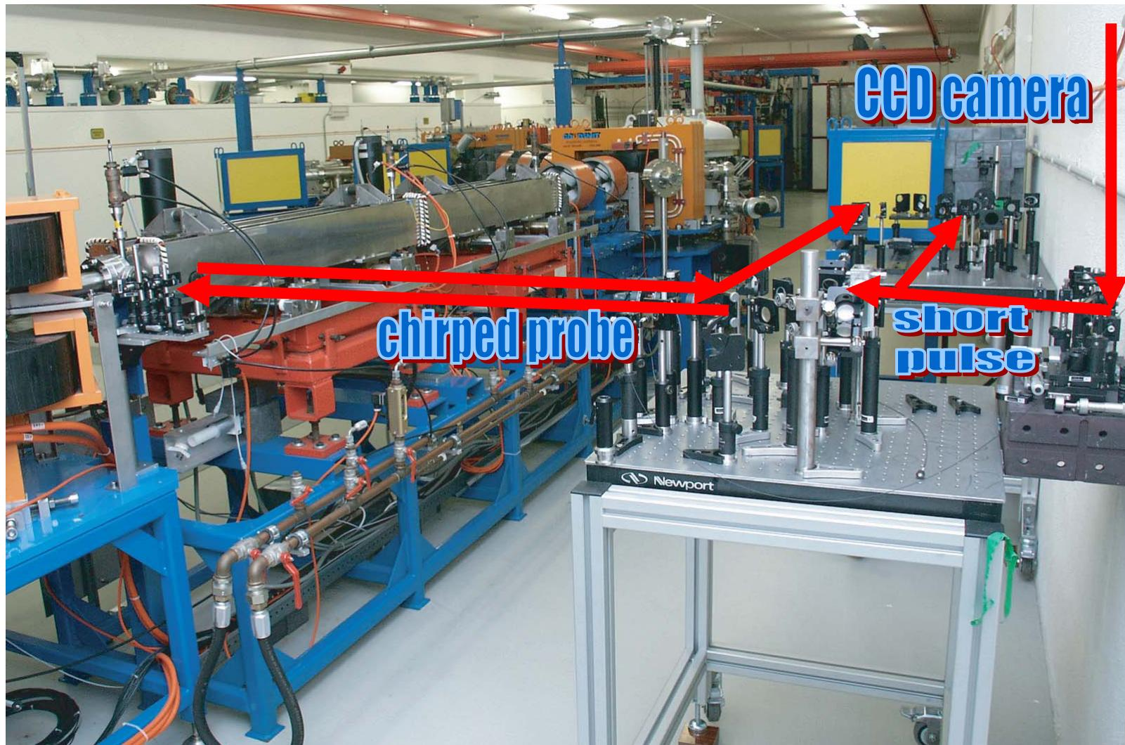
Electro-optic longitudinal beam-profile diagnostics,
