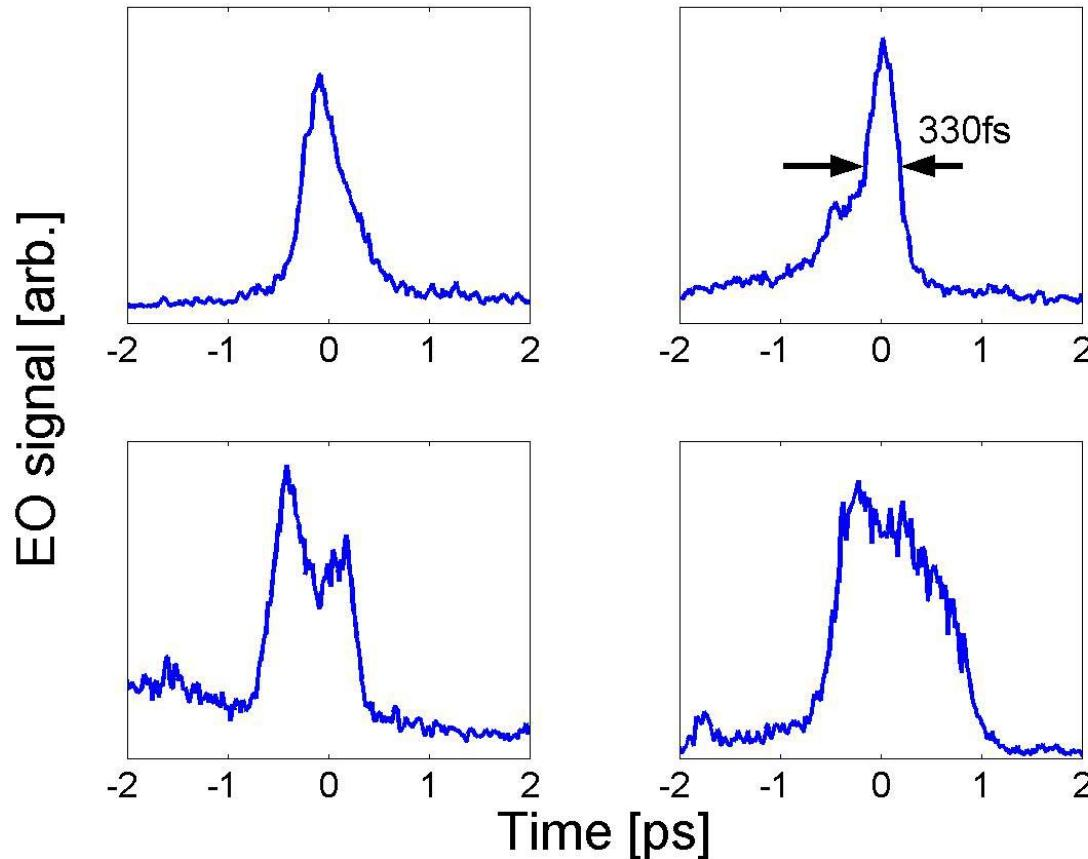
Bunch profile modified by changing the buncher and accelerator phase.
