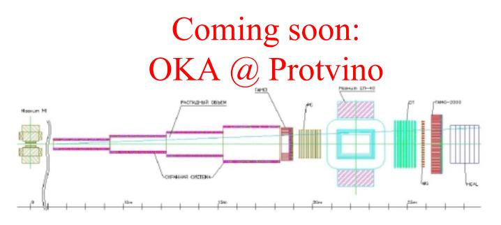
New RF-separated beam (CERN-Karlsruhe 1.2MV separators) at U-70 PS in construction: half of beam line ready, 3×10<sup>13</sup> ppp slow-extracted
