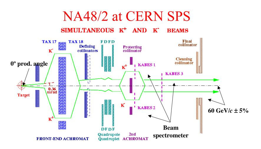
New *simultaneous* K+ and K- narrow band beam Kaon momentum spectrometer
