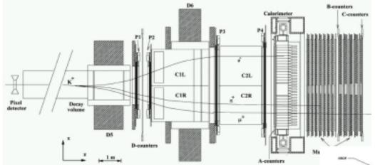
E865: completed 6 GeV/c Pixel+Cerenkov for K Spectrometer with dead region, Shashlyk calorimeter
