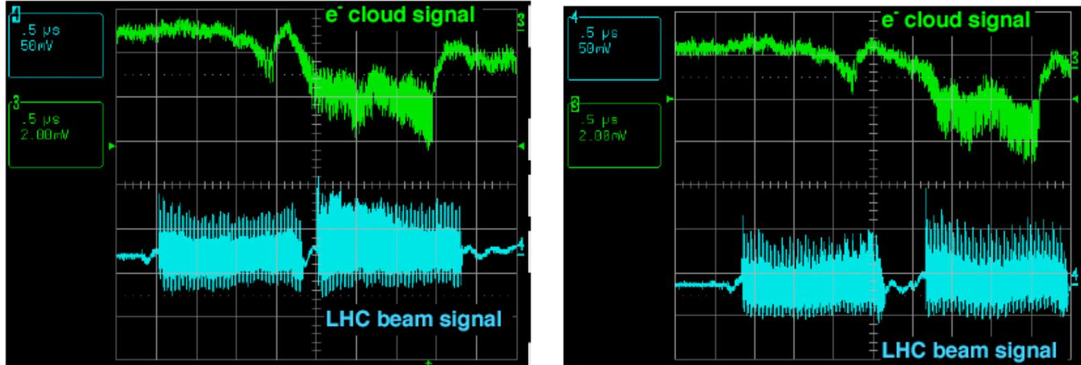
SPS pick-up signals for 225-ns and 550-ns spacing between two 72-bunch trains. Memory!
