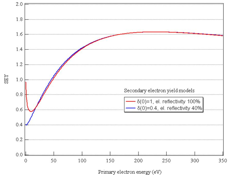
Fig. 1\_zoom. Details of the simulated SEY at low incident electron energy
