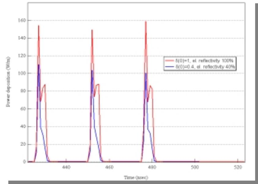
LHC field free region. Electron line density in electrons/meter and power deposition in W/m for three different reflectivity behavior at low incident electron energy. Note: CERN measurements by R. Cimino and I. Collins show 100% reflectivity at zero energy.
