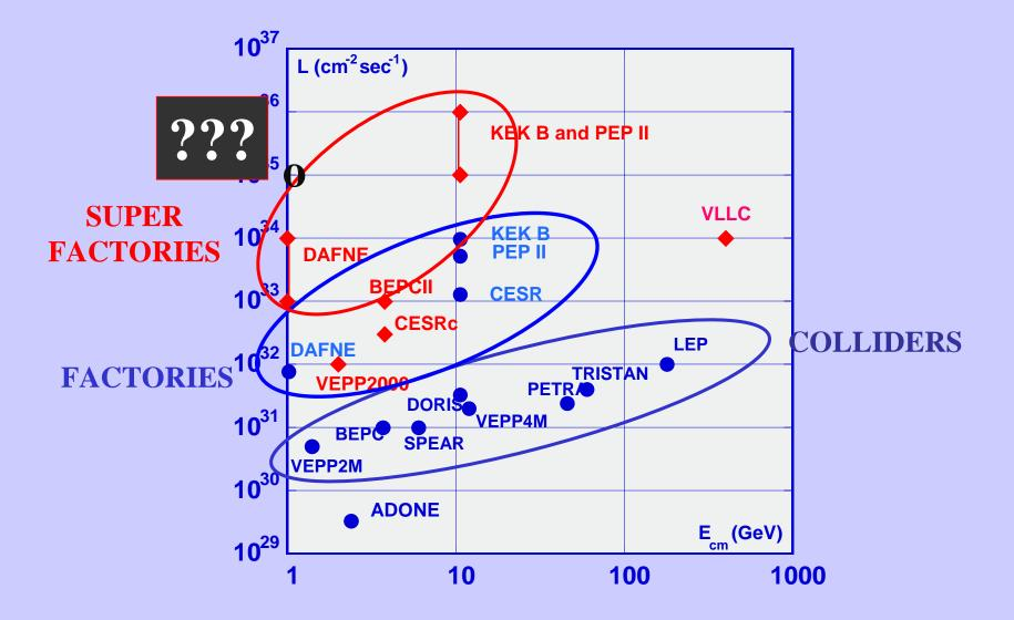
PEAK Luminosity increase total current and per bunch current increase n of bunches decrease beam sizes
