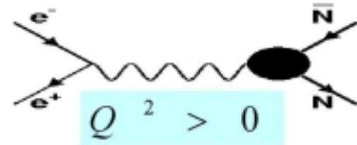
$$\frac{d\sigma}{d\Omega} = \frac{\alpha^2 \beta C}{4Q^2} \left[ |G_M(Q^2)|^2 (1 + \cos^2 \theta^*) + \frac{4m_p^2}{Q^2} |G_E(Q^2)|^2 \sin^2 \theta^* \right]$$
