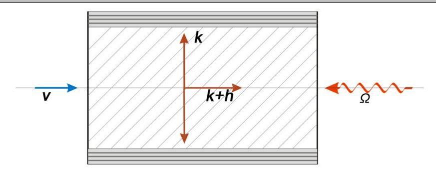
Wave **k** stands for the confinement of the radiation field inside the resonator; Wave (**k**+**h**) – for the beam modulation.
