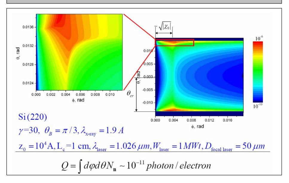
Intensity of the spontaneous radiation is **limited**. Further enhancement of the spectral density is possible using selfamplification on the expense of electron beam modulation at the feedback presence (SASE).
