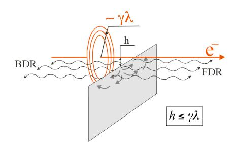
Diffraction radiation appears when a charged particle moves in the vicinity of a medium.
