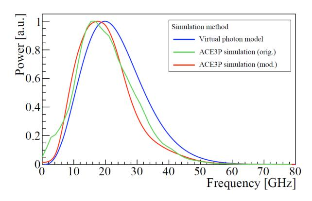
The normalized power spectrum from a 2mm Gaussian beam obtained with virtual photon model with the same parameters as for time-domain simulations (blue curve).
