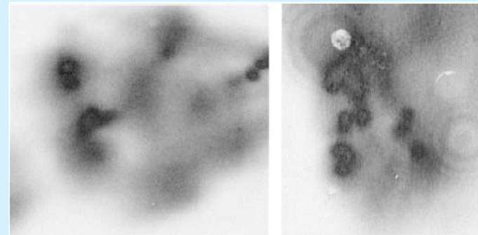
Filamentation of fs laser pulse along propagating length in dry air (left) and during the rain (right) (Mechain *et al.*, Appl. Phys. B, 80, 785 (2005)).
