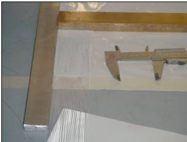
cladded scintillating fibers, Pol.Hi.Tech type 0046, 1 mm diameter
