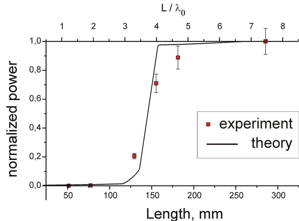
Dependence of radiation power on resonator length
