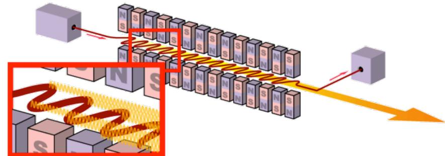
In an FEL a beam of relativistic electrons produced by an electron accelerator passes through a transverse, periodic magnetic field produced by a magnet called an undulator and exchanges energy with an electromagnetic radiation field.
