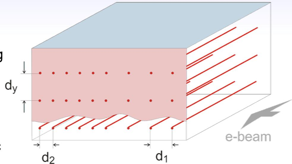
The "grid" structure is made of separate frames each containing the layer of 5 parallel threads with the distance between the next threads  $d_y=6$  mm), 12 frames were joined to get the "grid" photonic crystal with the period 12.5 mm and another 12 frames formed "grid" photonic crystal with the period 10.5 mm .
